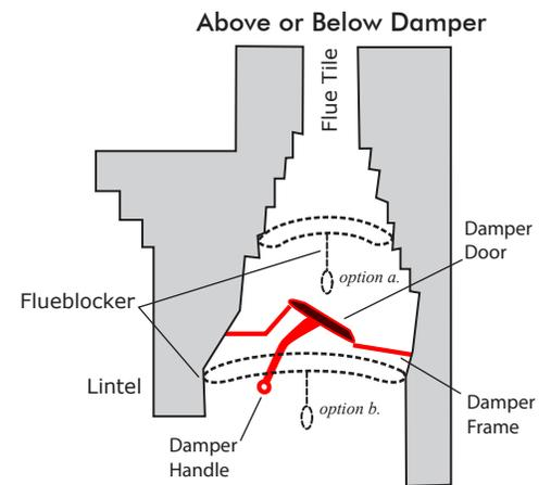
5. Obstructions like damper handles or cables can often be mitigated by removing the cotter pin or bolt holding it in place. If you can't remove the obstruction, open the damper and install the Flueblocker above the damper. Or you can also cut a hole or slit in the Flueblocker to accommodate the hardware, but this may affect the tightness of the seal.
